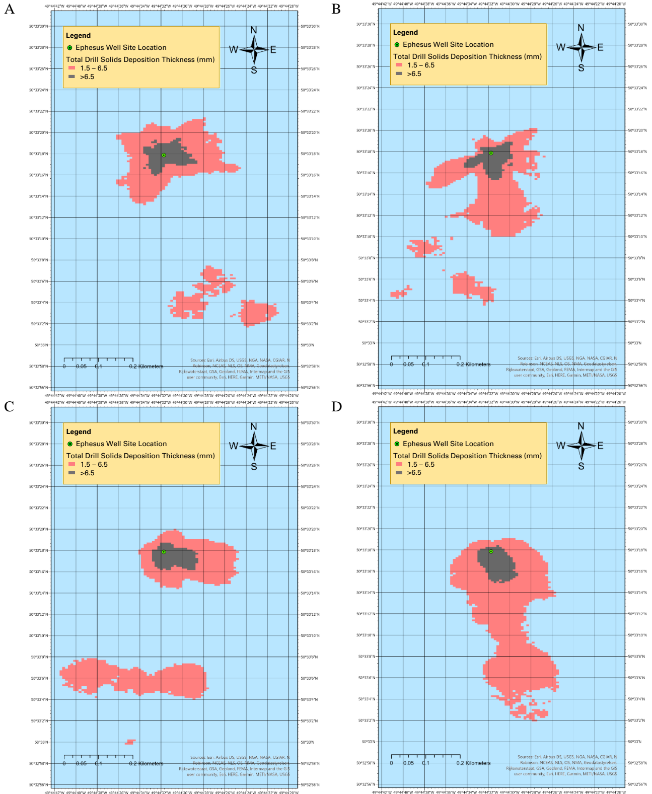
Figure 4-1 Predicted Drill Solids Deposition at the Ephesus well location after 75 days. A) Lowest Ambient Surface Current, B) Highest Ambient Surface Current, C) Lowest Ambient Benthic Current, and D) Highest Ambient Benthic Current (bp 2022d).
