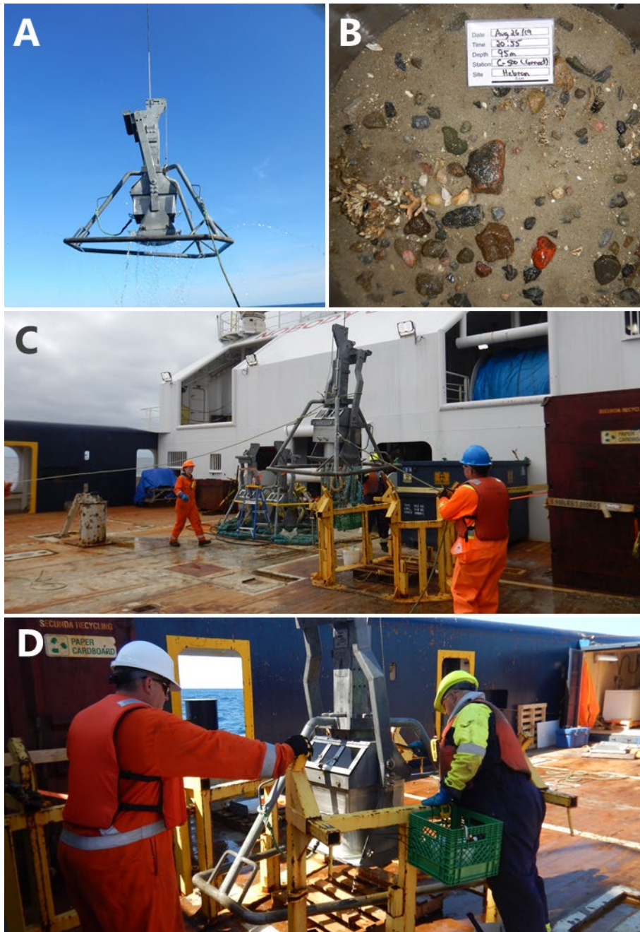
Figure 4-1 Sediment sampling operations, A) large-scale box corer, B) sediment sample example, C) sediment sample deck operations, D) sediment sampling.
