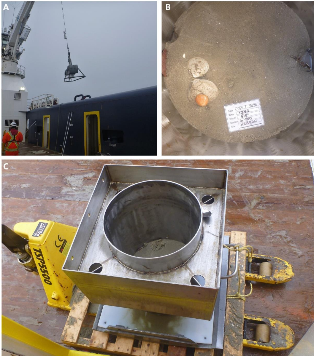
Figure 4-1 Sediment sampling operations: large-scale box corer (A), sediment sample example (B), sediment sample on deck (C).
