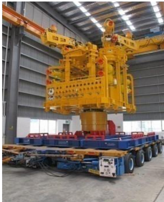
Figure 2: Typical capping stack device
