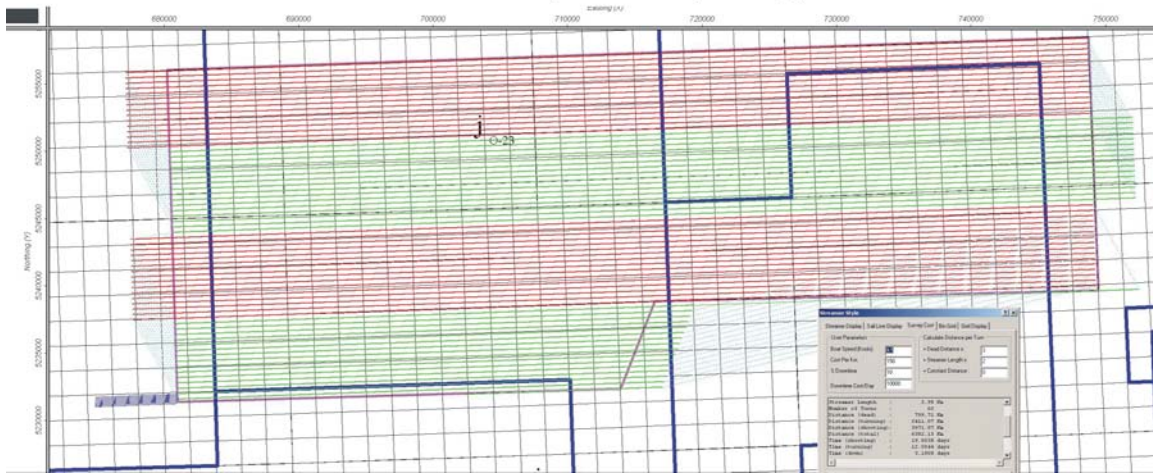
Figure 2. Proposed Sail Lines at 200-m and 400-m Separation. Actual separation distance will be dependent upon contractor selection.
