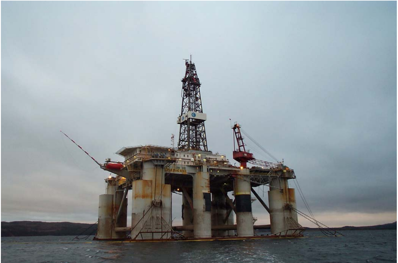
Figure 3.4 Typical Semi-submersible Drill Rig GSF Grand Banks .
