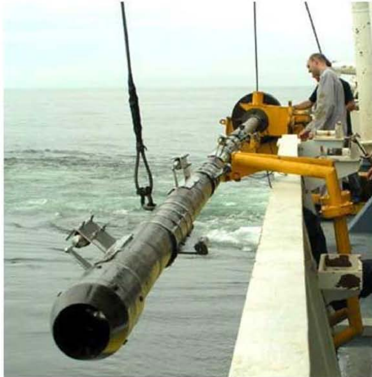
Figure 2-1 Thermistor (heat-flow probes) Outriggers on Gravity Coring System
