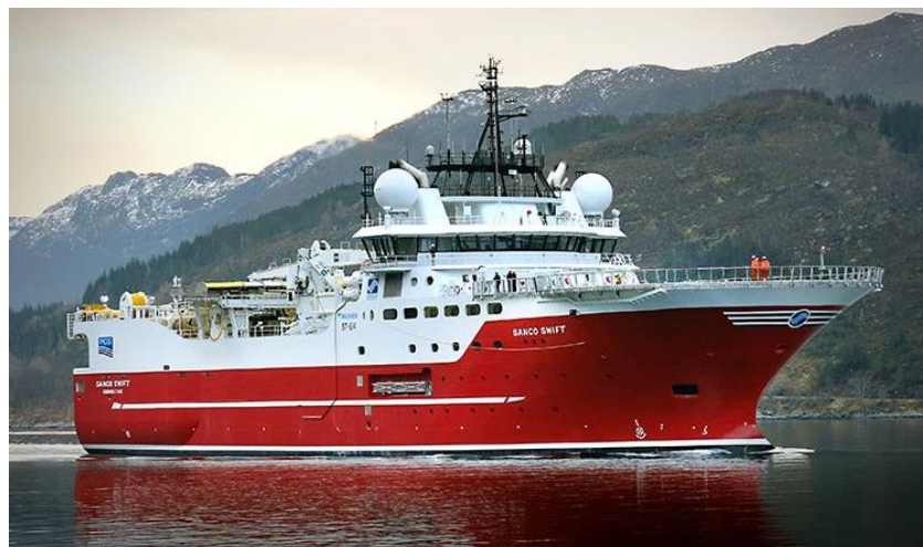
Figure 2.2. A representative 2D seismic vessel or source vessel for undershoots: MV Sanco Swift .
