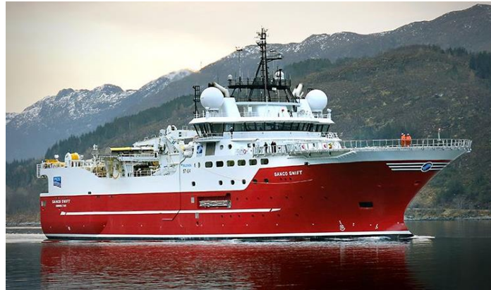
Figure 2.2. A representative 2D seismic vessel or source vessel for undershoots: MV Sanco Swift .
