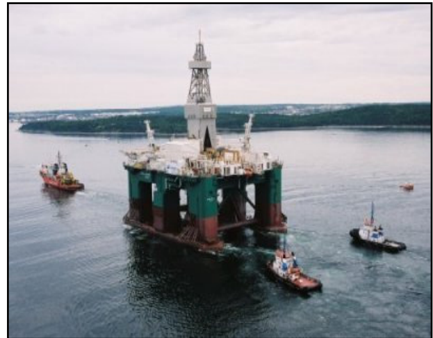
Semi-submersible Drilling Unit
