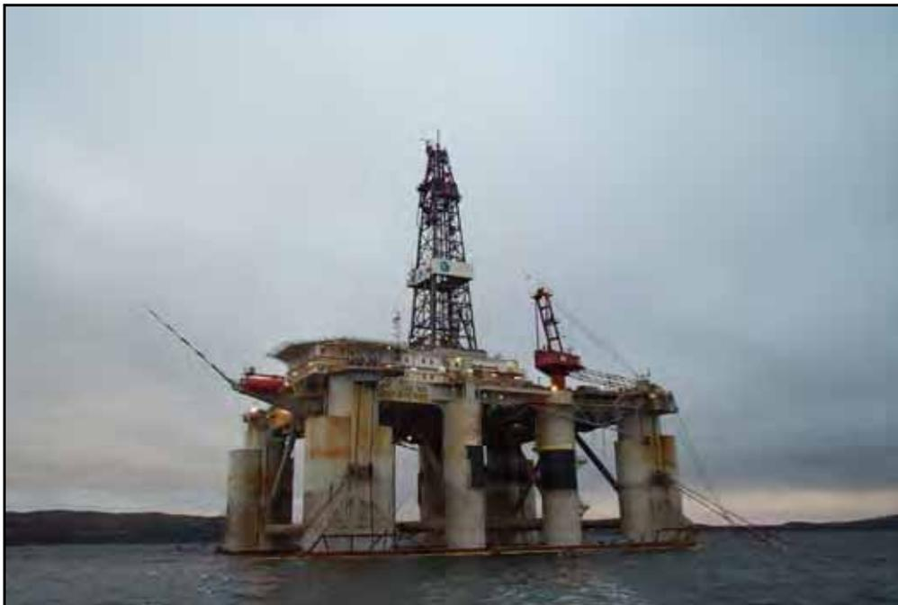
**Figure 4.5.** Semi-submersible Drill Rig *Glomar Grand Banks*.
