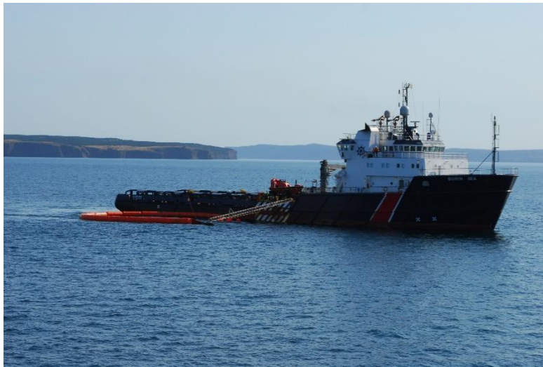
Figure 1. SVSS deployed from support vessel Source: CAPP
