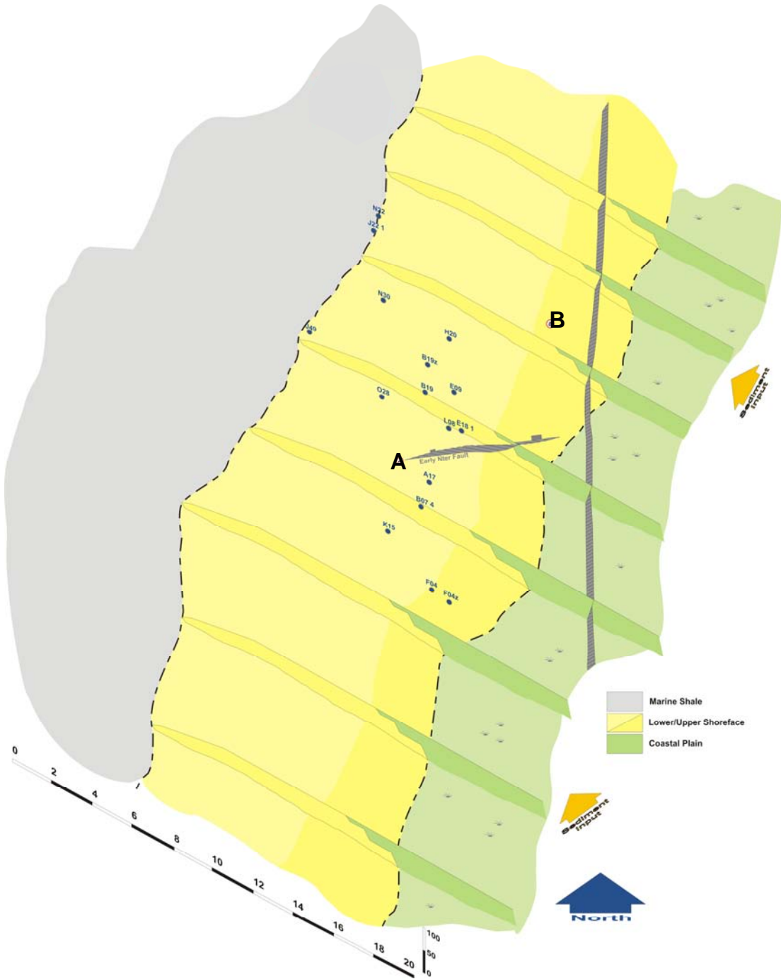
Figure 3.2 - Schematic of Aerial Distribution of Shoreface Sandstone and Early Moving Faults Related to the Initial Phases of Ben Nevis Fm Deposition (Note development wells are not displayed)
