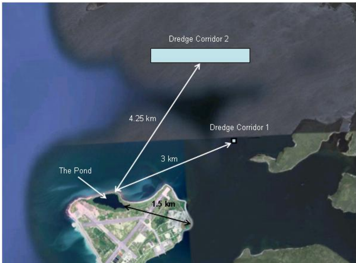
Figure 3-4 Corridors Requiring Dredging along the Concrete Gravity Structure Tow-out Route
