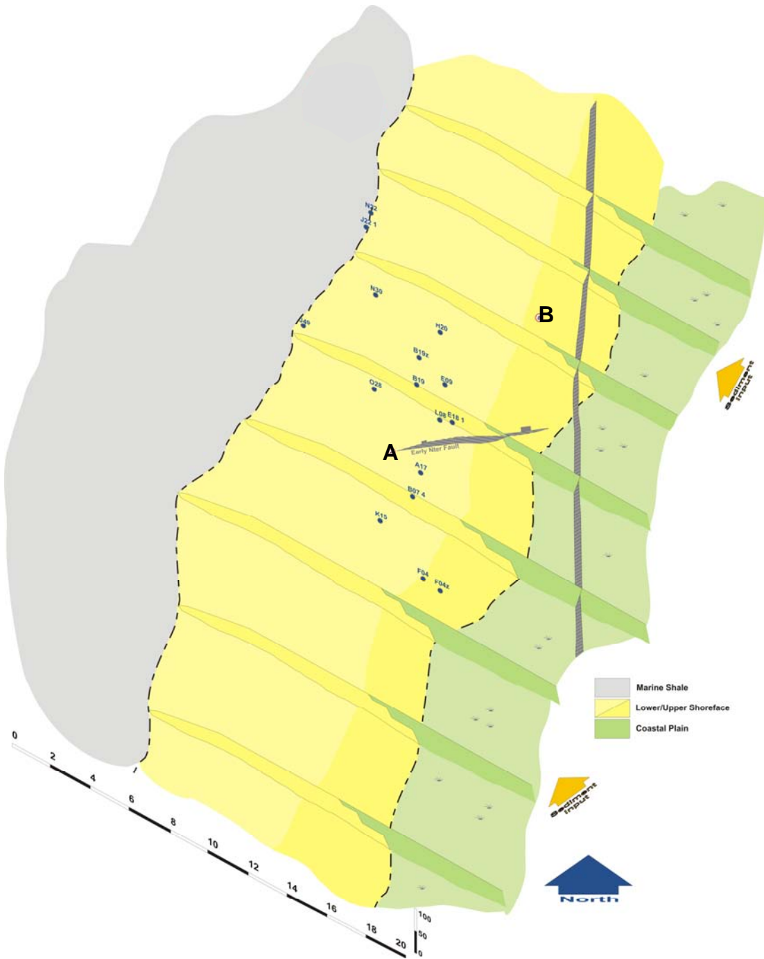
Figure 6.3 Schematic of Aerial Distributing of Shoreface Sandstone and Early moving Faults related to the initial phases of Ben Nevis Fm Deposition (Note development wells are not displayed)
